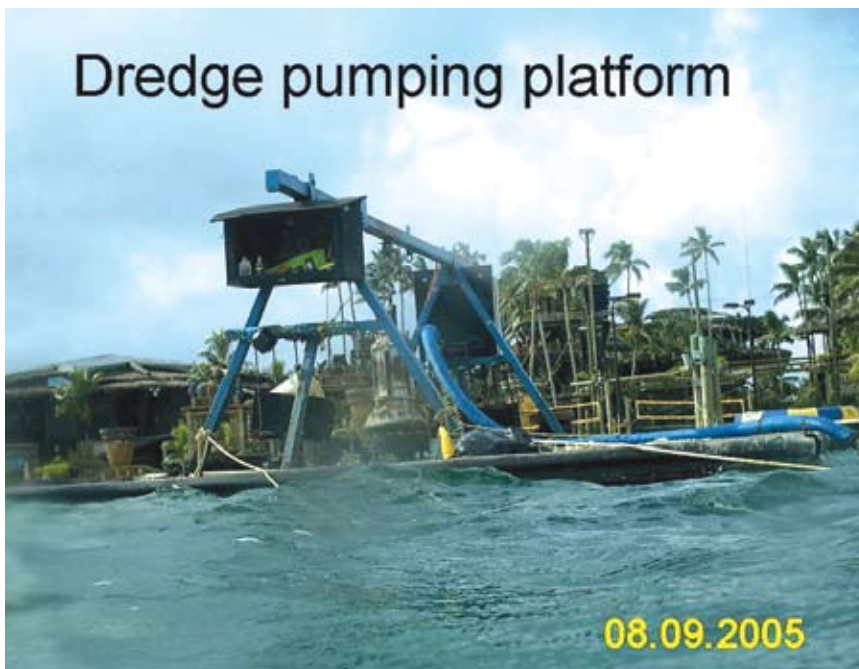
∧ ∧ ∧ “A floating platform was used to support a pump to move sand from offshore to the beach” (2005 Coastal Incident Report).
